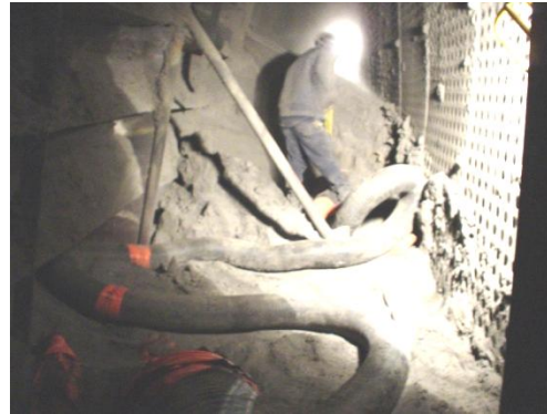
Inlet Turning Vane and Nozzle Pluggage
